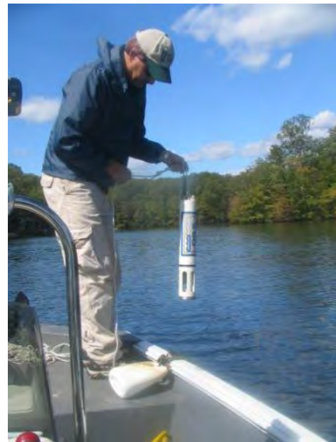
A water scientist uses a sonde for specialized testing.
