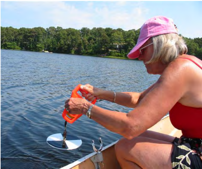
A volunteer sampler deploys a Secchi disk to measure water clarity.
