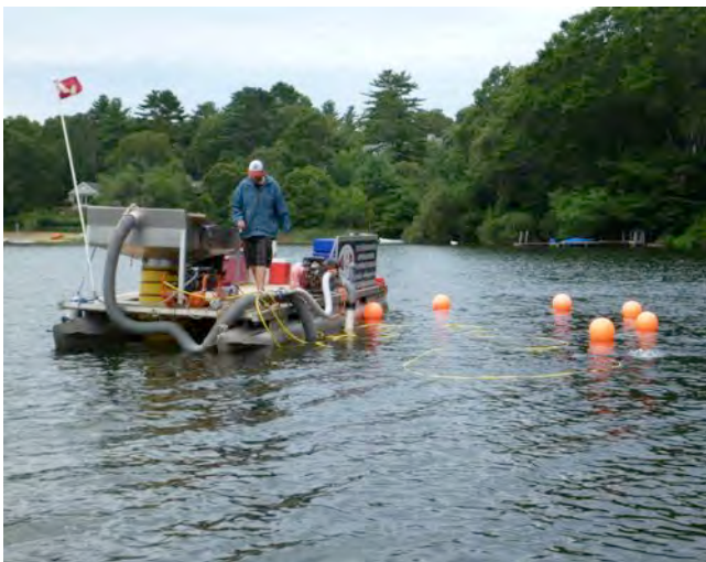
The DASH rig: pontoon boat with the diver submerged at the right where the bubbles are. The 6-inch suction hose is suspended from the orange floats. The small diameter hose on the water surface is the diver's air line.
