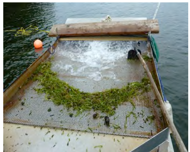
The suction hose discharges water and harvested Hydrilla into this perforated tray where the Hydrilla is loaded into plastic tubs for disposal.
